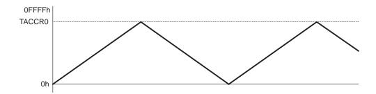
The count direction is latched. This allows the timer to be stopped and then restarted in the same direction it was counting before it was stopped. If this is not desired, the TACLR bit must be set to clear the direction. The TACLR bit also clears the TAR value and the TACLK divider.
